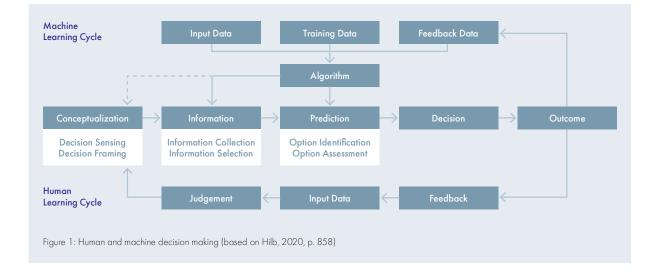
Figure 1 illustrates that both approaches – human and machine – to decision making assume that decisions are based on predictions of possible outcomes. In both approaches, predictions are based on some sort of input data which are then further processed to generate an output, i.e., the final decision outcome.
